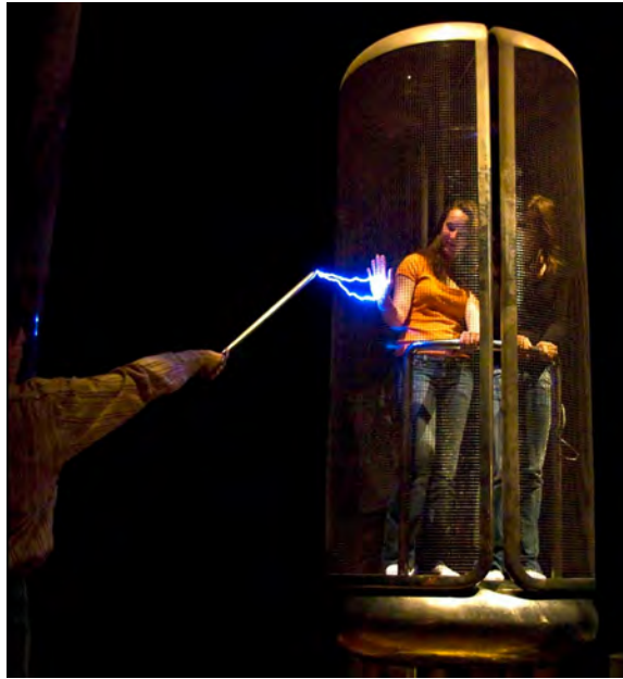
Figure 32.4: Faraday cage demonstration on volunteers in the Palais de la Découverte in Paris (courtesy of Wikipedia). When the cage is grounded, the potential at the surface of the cage is zero. By the solution to Laplace's equation, the potential inside the cage is a constant. Hence, the electric field inside the cage is zero. Charges will surge from the ground to the cage surface to make the potential zero inside the cage. Therefore, a grounded Faraday cage effectively shields the external fields from entering the cage.
