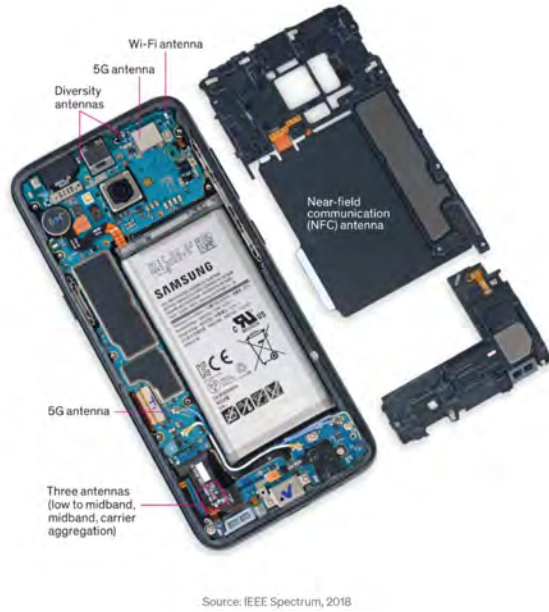
Figure 32.1: The compact locations of the cell phone components make urgent use of EMC/EMI knowledge instrumental in the design of cell phones. Clever use of shielding is necessary to prevent interferences between different components. Compatibility means that even when each component works well in isolation, but when brought to work alongside each other, they fail to work together.
